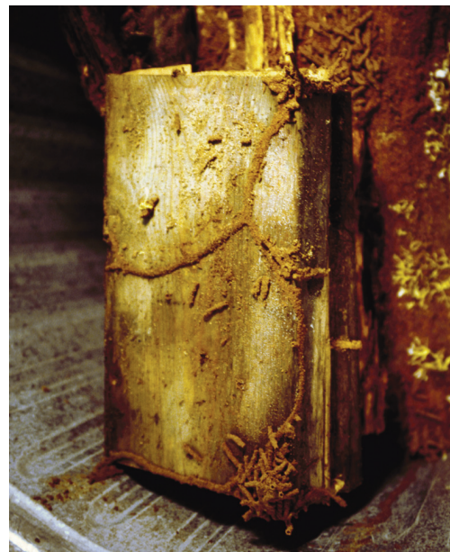
Figure 16. Warm, moist wood provides subterranean termites with all of their survival requirements.
