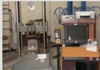
Satec machine with Instron electronics configured to test furniture frame joints. 60(kip).
