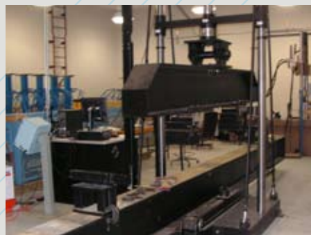
Universal Testing Machine with a 24 foot bed. 130(kip).
