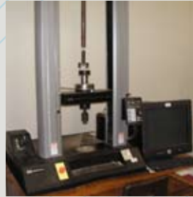
Instron tabletop testing machine for MOE, MOR, and IB. 2(kip).
